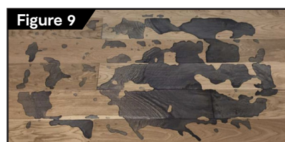
30-Hour Standing Water Test Assembly at the 24-hour mark
